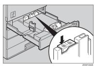
While pressing the release lever, adjust the back guide to the new paper size.
